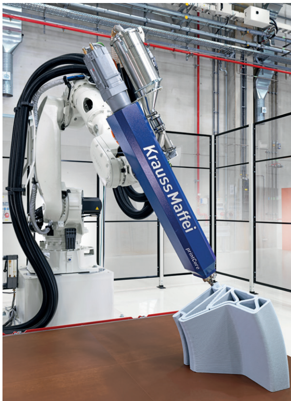
powerPrint Flex – a highly flexible, powerful system for industrial additive manufacturing with a robot.
