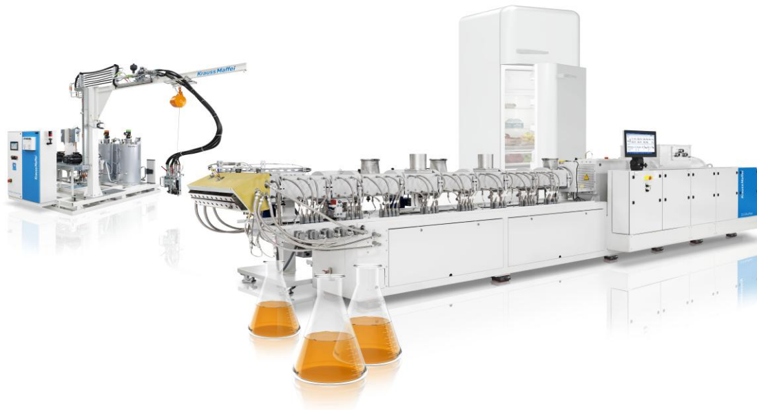
Figure 5: Twin-screw extruder ZE BluePower for the depolymerization of polyurethane into recycled polyol
