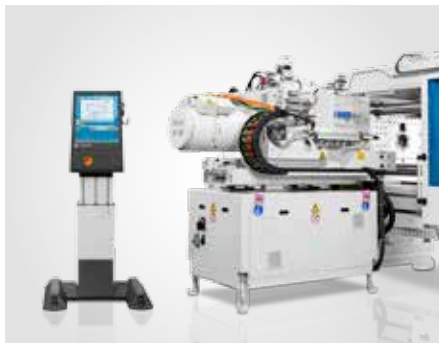
The all-electric version meets demand for extreme shot weight consistency for high-precision applications.
