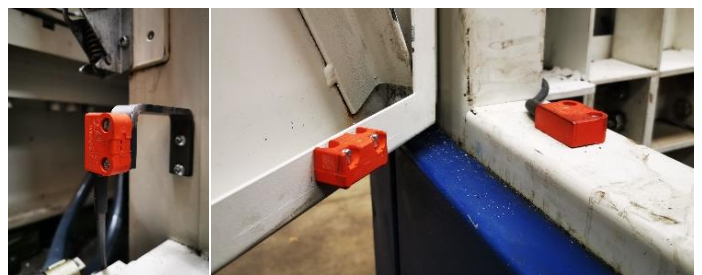
Examples of the emergency stop 2-channel safety concept with contactless circuit breakers on all door elements
