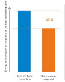
Up to 30 percent lower energy consumption by the pump of the heat-balancing units with the use of new water distributor.
