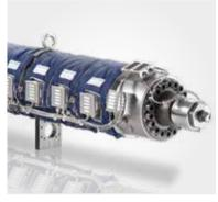
**Full insulation for plasticizing barrel** A precisely fitting sleeve of multilayered glass fleece sewn into a protective fabric significantly reduces energy consumption. The insulating sleeves sustainably reduce radiation losses from the heating tapes to the environment.
