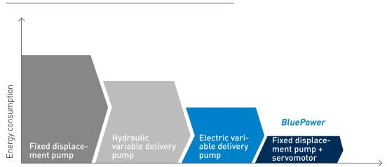
Minimum energy consumption with the BluePower Vario Drive Comparison with other pump systems
