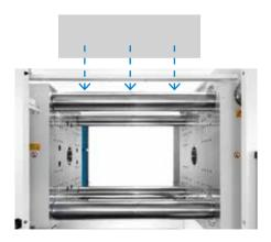
Even complex molds can be installed simply by removing the bar. The mold can even be introduced laterally for low shop heights.
