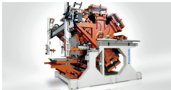
Drum unit equipped with two robotically manipulated mixing heads to enable quick filling of doors for increased productivity.
