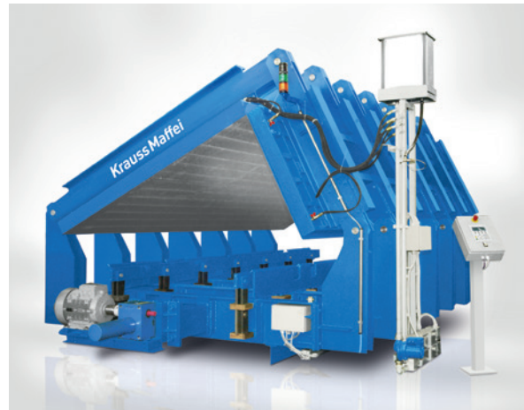
Triangular fixture for the production of commercial refrigerators.
