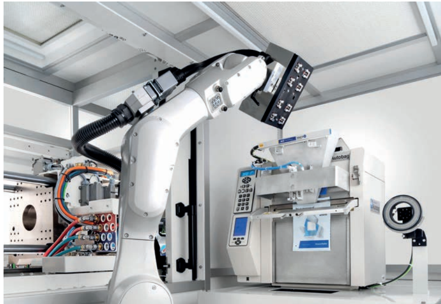
Fig. 1. Compact automation system with its own laminar flow box, packaging station and camera for parts inspection © KraussMaffei
