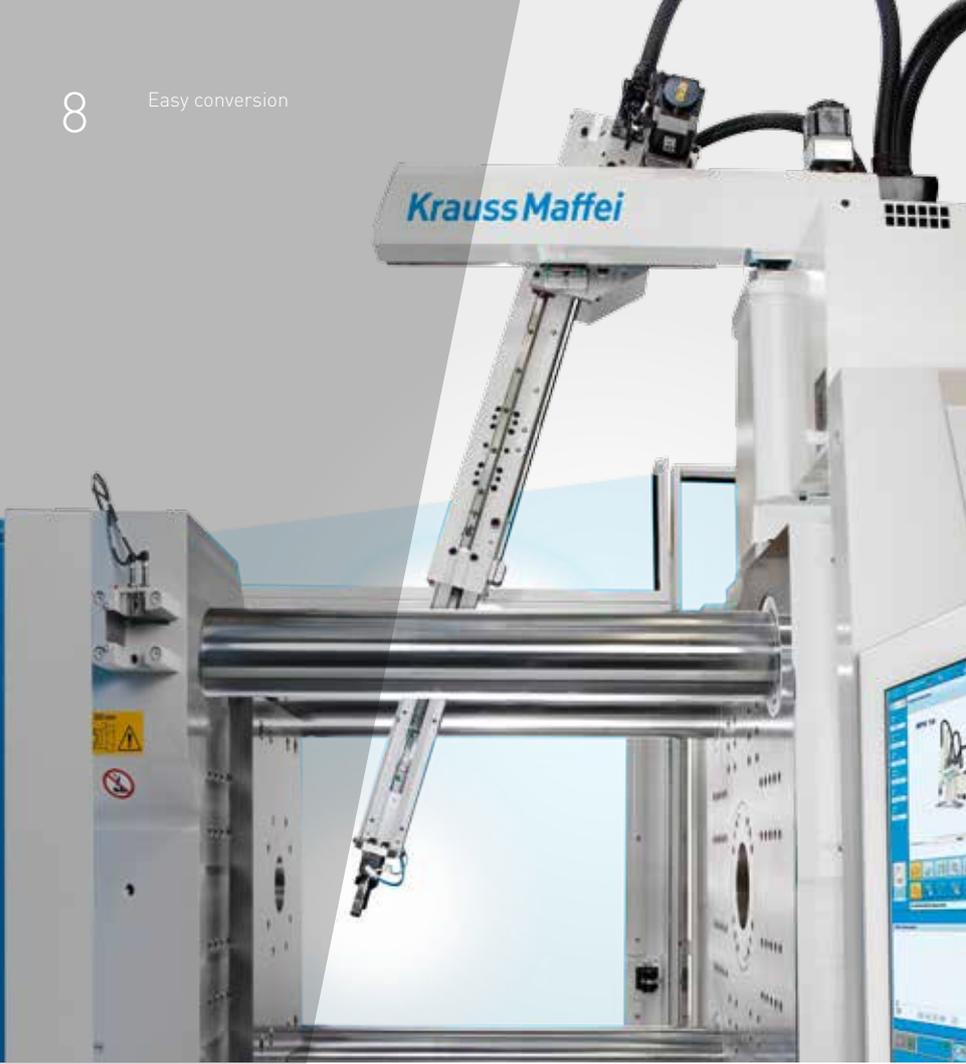
The one-of-a-kind inclined position of the Y-axis provides flexibility across the full range of clamping forces - regardless which product you are demolding.
