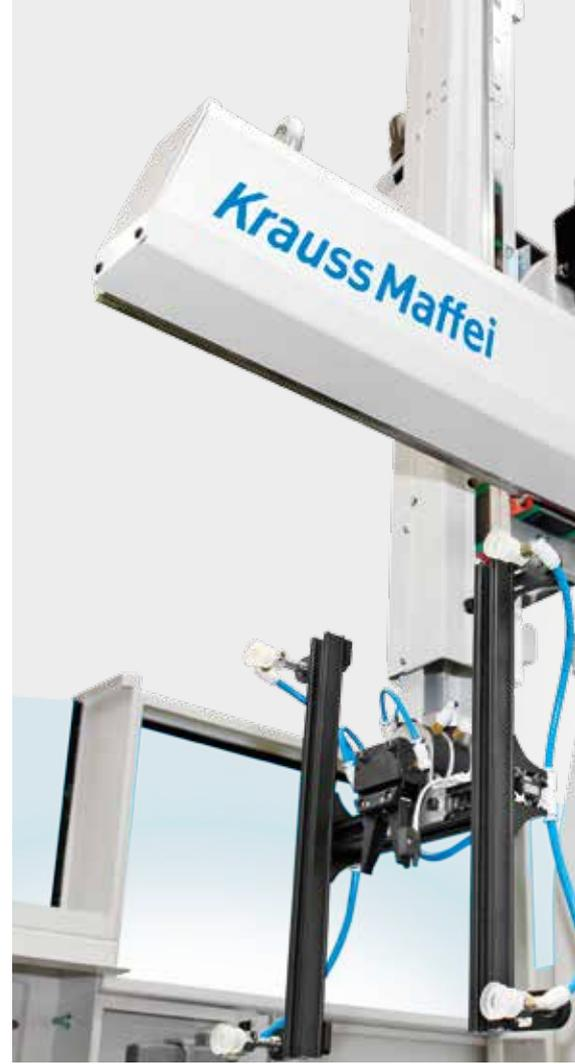
With the optimal gripper module, the SPX10 can demold and deposit even small parts using vacuum.
