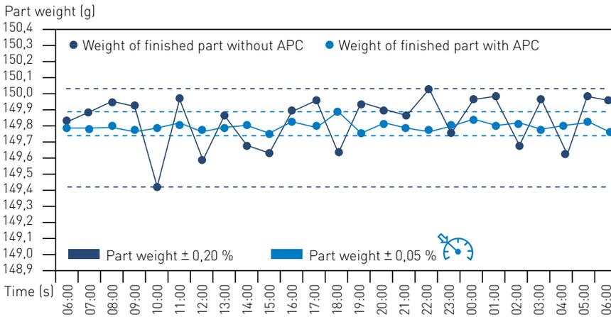
This graphic illustrates fluctuations in component weight, which are greatly diminished when APC is used. This improves the process capability significantly and reduces the expected scrap rate substantially.
