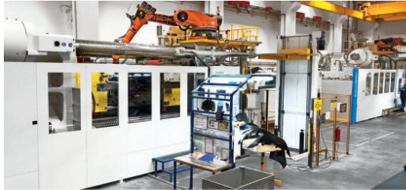
A total of four KraussMaffei MX machines form the foundation for the production of bumpers at the plant in Bursa
