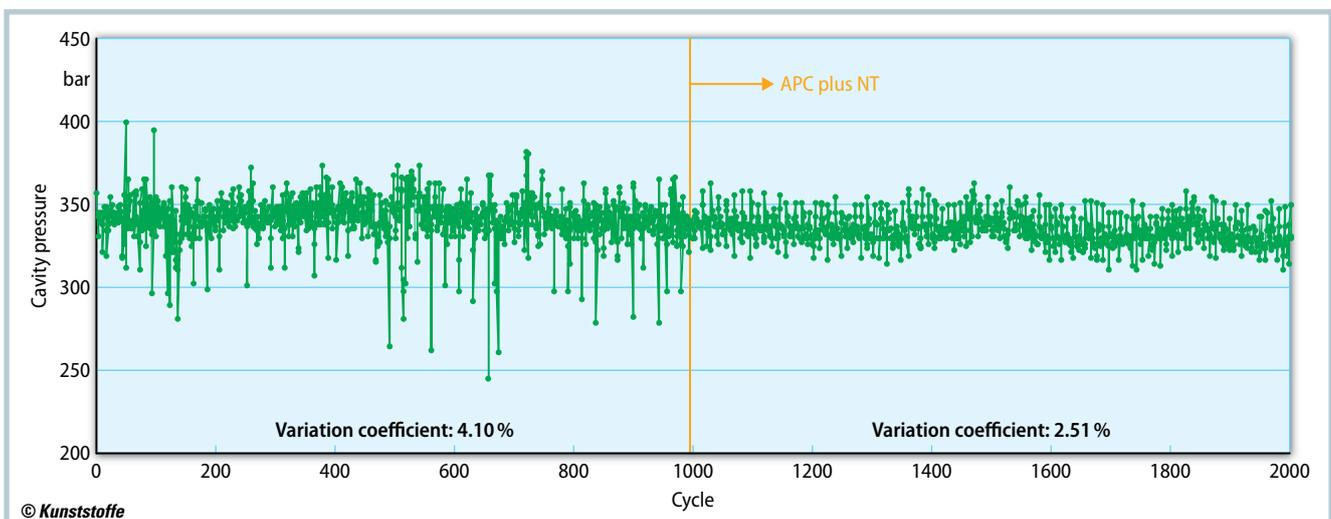
**Fig. 2.** A 48-hour test (24h without and 24h with APC plus) shows that the machine function significantly reduces the fluctuation band of the cavity pressure (NT = non-thermoplastics) (source: KraussMaffei)
