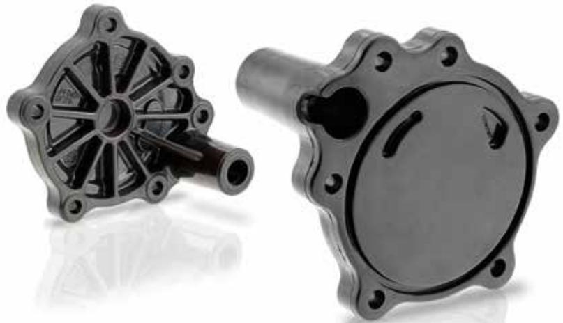
Key to the vacuum pump cover is the absolutely flat functional surface (right). The challenge here is that the pronounced rib structure on the reverse side (left) must not show through on the flat side. This can be solved by using PF thermoset compounds (© KraussMaffei)
