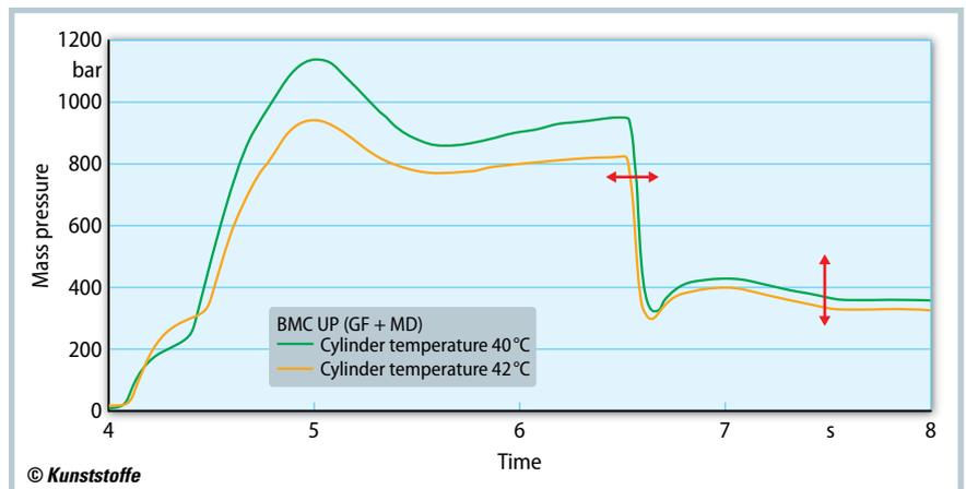
**Fig. 4.** If the cylinder temperature rises by 2°C, and the mass becomes less viscous, APC plus switches to holding pressure at an earlier point and reduces the pressure level to prevent over-filling of the part (source: KraussMaffei)
