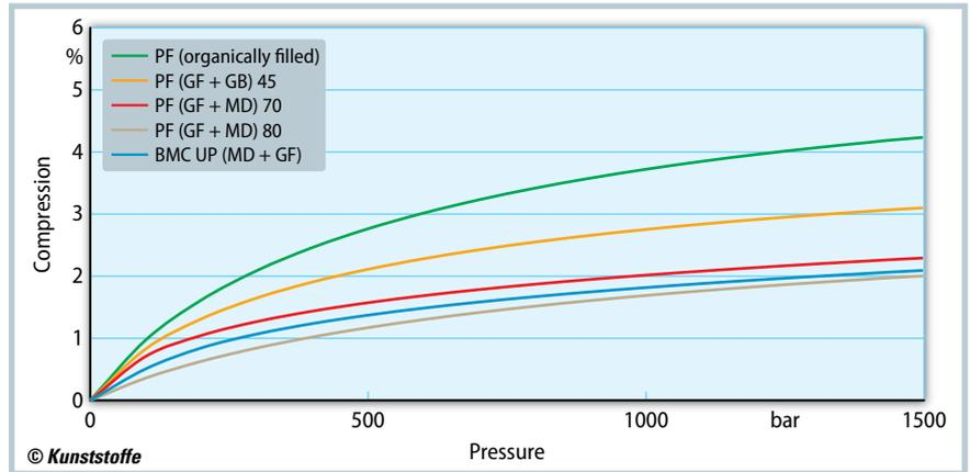
**Fig. 3.** The more highly filled, the lower is the material-specific compression curve. At 1000 bar pressure, the mass column of an organically filled PF is compressed by 3.7%; at 80% filling of glass fibers and mineral components, it is only 1.8% (source: KraussMaffei)
