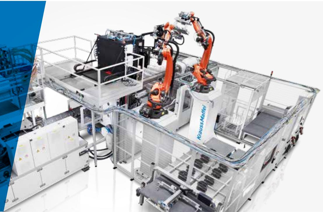
FiberForm technology from KraussMaffei combines thermoforming of thermoplastic semifinished products with injection molding. All FiberForm production systems from KraussMaffei have a modular design. Product-oriented automation solutions ensure efficient manufacturing.
