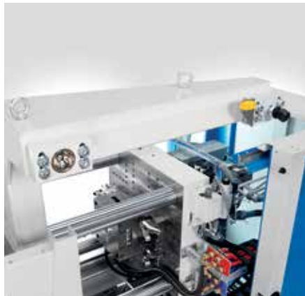
Docking console on the injection molding machine
