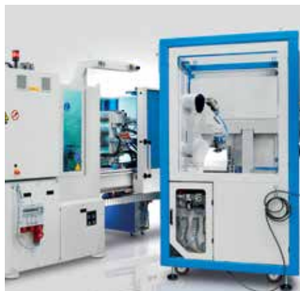
Easily accessible connecting lines – “plug-and-play”
