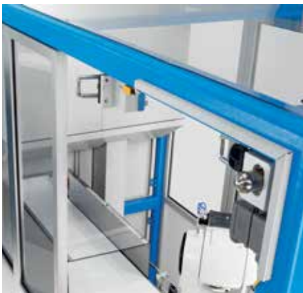
Docking console on the cell's base frame
