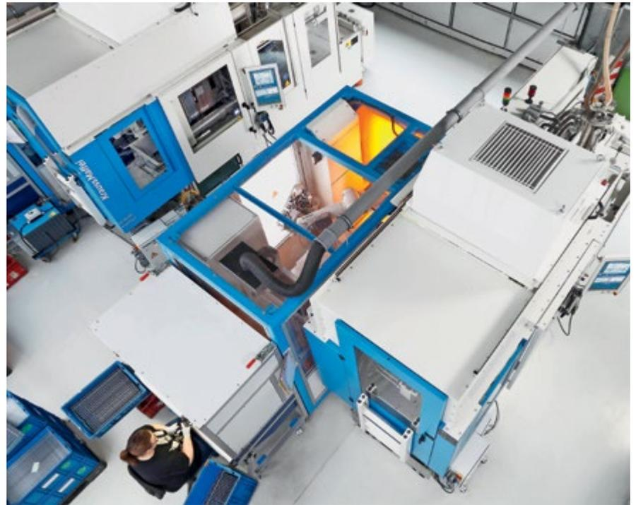
**Flexible Automation:** Thanks to dockable automation, use of the injection molding machine – with or without automation – is just as possible as relocating the cell to another site of production. Thus, maximum flexibility when changing products or molds is provided. Photo: Krauss Maffei
