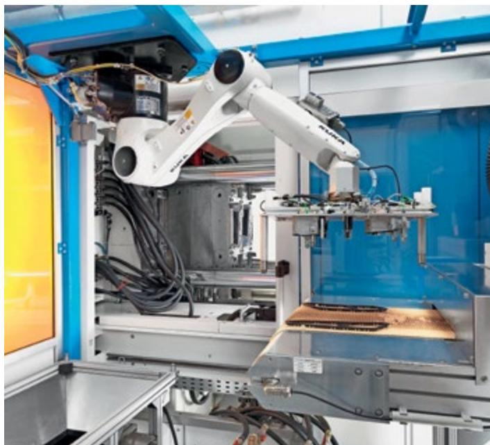
**Integrated and space-saving:** The hanging 6-axis robot with article specific gripper ensures safe and secure handling as well as film curing in the UV tunnel. Photo: Krauss Maffei
