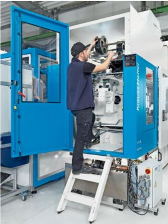
**Space-saving and ergonomic:** The CX 160 offers excellent accessibility for changing film rolls. The entirety of film peripherals (spool core, control unit) can be integrated below the cantilevered clamping unit.
