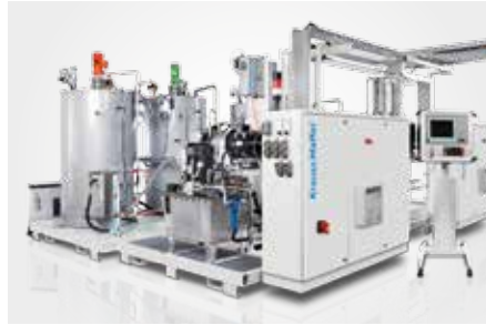
RimStar Compact 40/16 metering machine for supplying a maximum of 8 mixing heads
