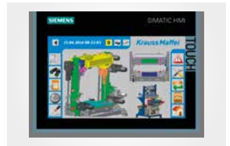
Intuitive operating software for programming mold carrier movements and mold functions without the need for prior knowledge of programming
