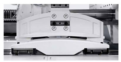
The GuideX guide shoe absorbs forces and protects the guides. This ensures that the linear guide maintains its ease of movement and precision over the long term.
