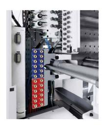
All of the important interfaces for the mold can be reached easily.
