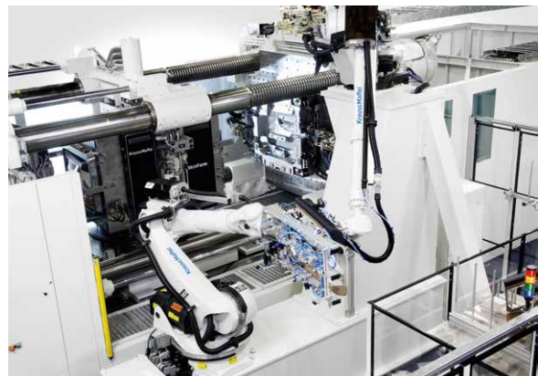
MX series designed as three-component SpinForm technology (swivel plate).
