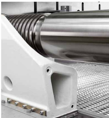
The force flow and weight-optimized sliding shoes ensure that the moving platens are guided securely.
