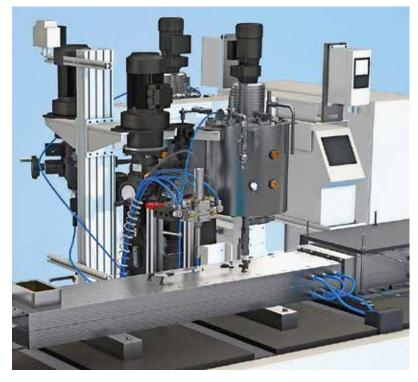
The process of soaking the fibers with the matrix material takes place directly and continually in the injection box. This allows systems with higher reactivity to be processed. These systems can be selectively configured to match the property patterns of the end product.
