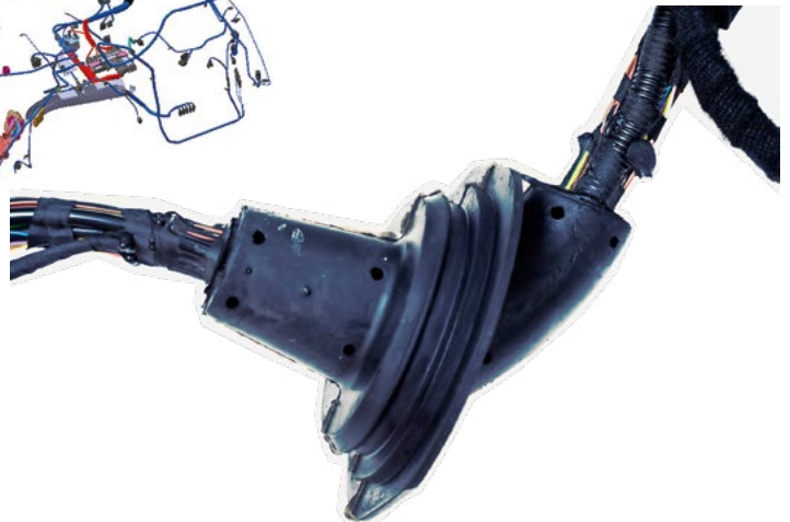
Figure 2: The polyurethane foam reliably fills the intermediate spaces in the cable harness, which means that no moisture can ingress into the vehicle's interior. Furthermore, the elastic polyurethane material also ensures secure assembly in the grommet fitting.
